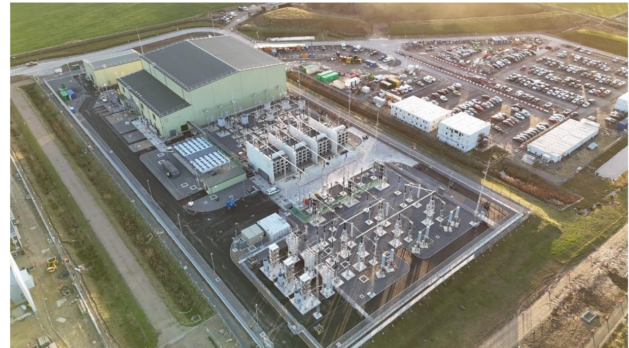
Plate 2-20 Example Onshore Converter Station (Source: Dogger Bank C)
